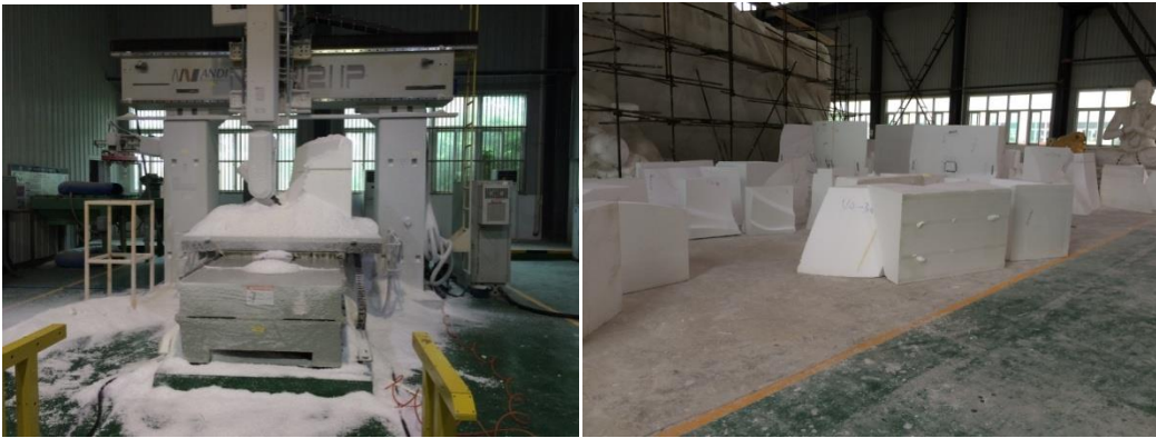
Manufacturing of foam model with CNC machine
