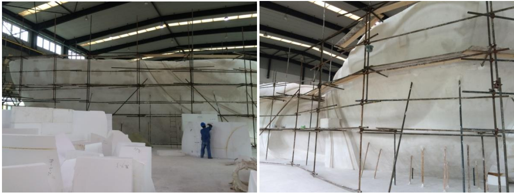
1:1 body part 1:1 foam model assembly and modification
